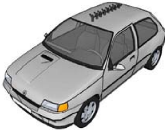
Figure 4.18 – Linear phased array mounted on the roof of a car
