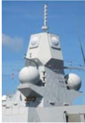
(b) Naval Radar: Thales APAR [6]
